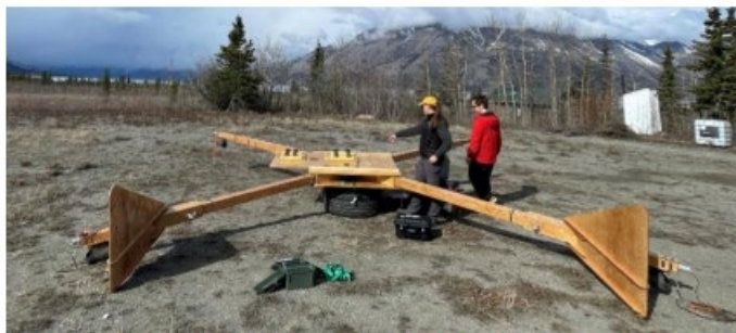
The AirlPR system set up and ready to measure the ice thickness of glaciers in KNPR
